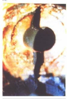
3. Trust your eyes. An example of the significant cracking along the inside diameter of the header, as revealed by a borescopic inspection. Courtesy: Thielsch Engineering Inc.
